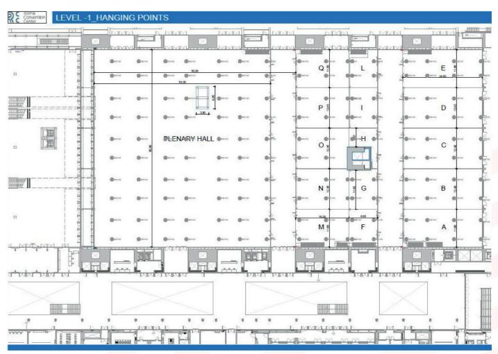
Each point has a maximum load of 500 kg. For all suspended loads installed by the user, subject to authorization by the Roma Convention Center Technical Department, a special calculation report and verification of the entire structure (from the hooking point to the spotlight) and all components that contribute to the rigging (motor, hook, truss cable, etc.) must be prepared at the user's expense and care, and signed by a qualified technician compliant with Min. Int. Circ. No. 1689 of 1/4/2011.
