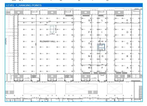
Each point has a maximum load of 500 kg. For all suspended loads installed by the user, subject to authorization by the Roma Convention Center Technical Department, a special calculation report and verification of the entire structure (from the hooking point to the spotlight) and all components that contribute to the rigging (motor, hook, truss cable, etc.) must be prepared at the user's expense and care, and signed by a qualified technician compliant with Min. Int. Circ. No. 1689 of 1/4/2011.
